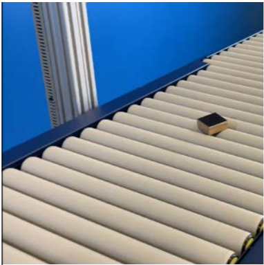
Measure Cuboidal and Irregular Shaped Parcels Approved on small items down to 20mm height for cuboidal and irregular objects of known shape.
